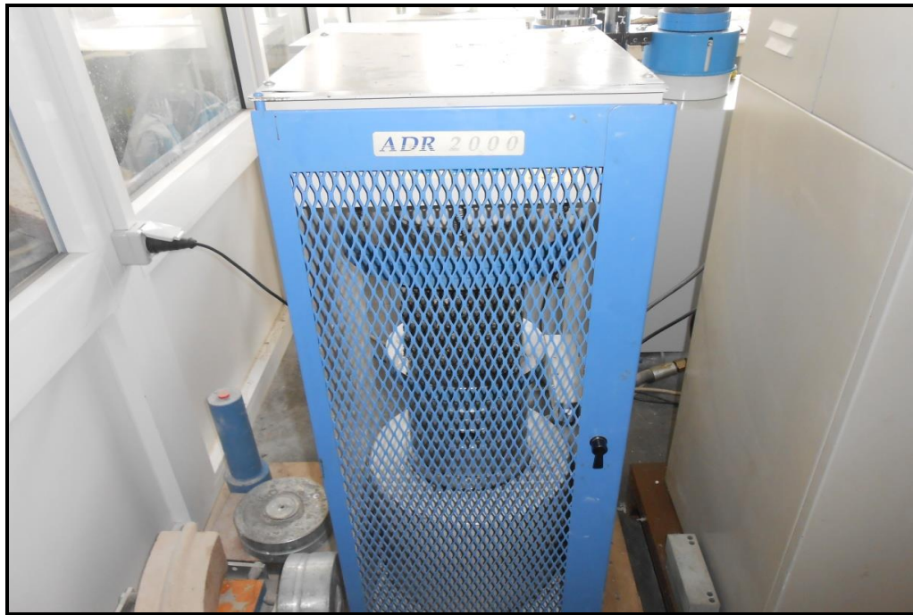
Figure 3.7: Apparatus of compression test.
