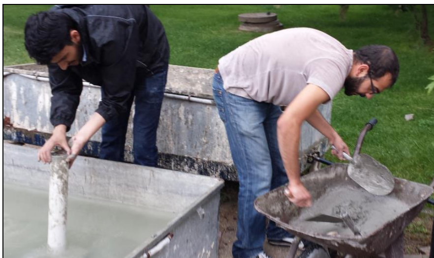
Figure 3.10: Pouring of underwater concrete
