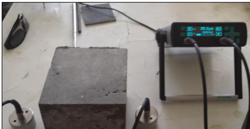
Figure 3.6: Apparatus of pulse velocity test.
