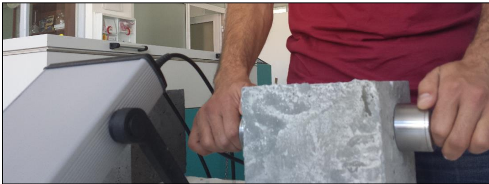
Figure 3.5: Application of pulse velocity test.
