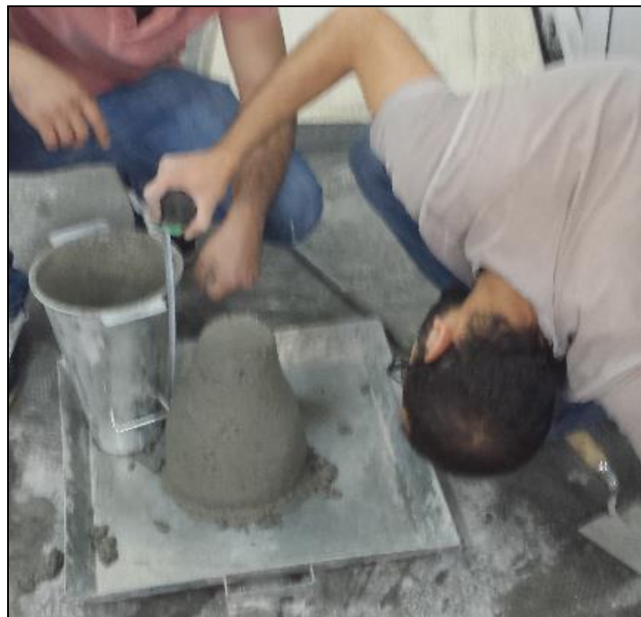
Figure 3.4: Slump cone and testing.
